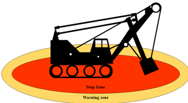
FIGURE 10.18 Shovel equipped with proximity detection system.
